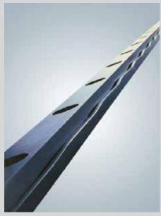
Due to the elastic deformation from both the upper and lower beams of the press brake during the ben ding process, the bending angle is not constant over the entire bending(plate)length. The CNC-controlled crowning device compensates for is deformation so an equal bending angle is obtained over the full bending length.
