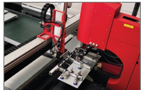
D: Inserting up to 6 different pieces of hardware in 1 single pass in both sides of the workpiece.
