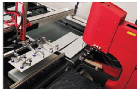
G: Stacking parts on the transport belt.
