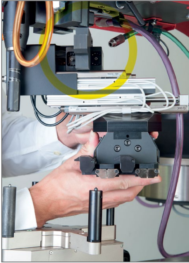
Dual station removed.
