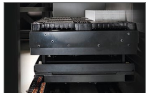
C: Automatic loading of a pallet of workpieces.
