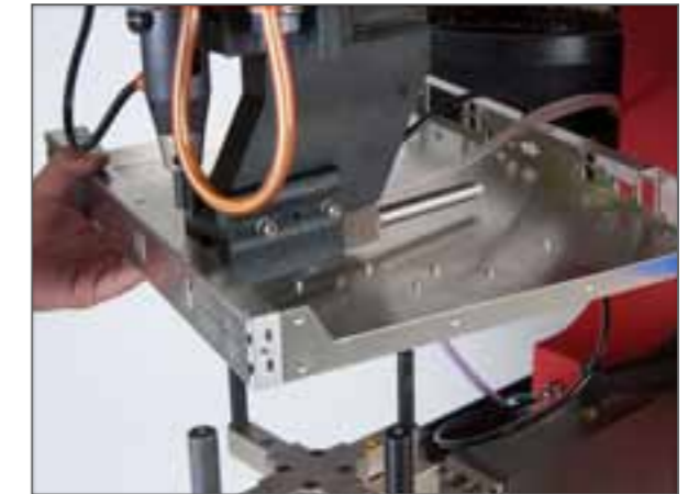
ABFT J-Frame for the difficult to reach flanges
