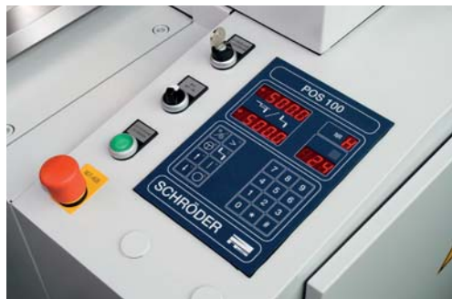
NC positioning gauge POS 100 with 9-step program 750 mm or optionally 1,000 mm
