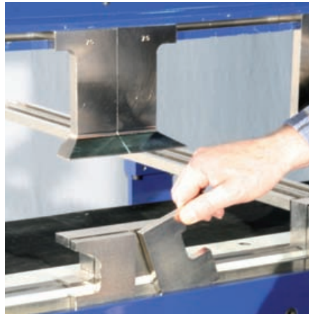
Patented eccentric fast clamping for the clamping and folding beams
