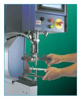
variables such as dwell time and installation force and automatically alert and direct the operator to any safety or system faults for quick diagnosis.
