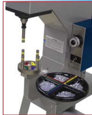
Round turret installed on an LT/4 press.
