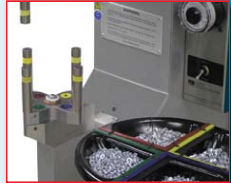
Star turret design for fastener-type installations that are more difficult to access.
